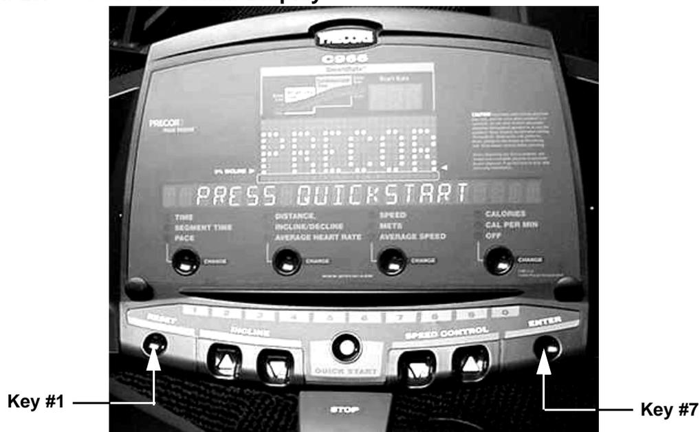
6. The keyboard test will place two dots on the display for each key on the display, including the numeric keypad. Pressing a key will cause the upper of the two dots associated with the key to go out. Test all of the keys in this manner. Tug on the safety key lanyard, to ensure that the **STOP** key is operating normally.
